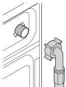
In order to prevent water leakage that may occur at the connection points, there are rubber seals (4 seals for the models with double water inlet and 2 seals for other models) attached to the hoses. These seals should be used at the tap and machine connection ends of the hoses. The plain end of the hose fitted with a filter must be attached to the tap and the elbowed end
